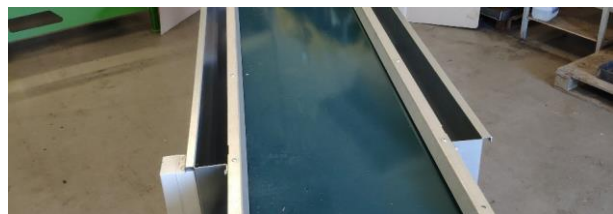
waste lanes on the upper side of the belt
